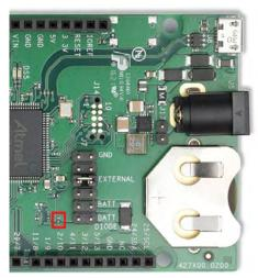
Figure 5: Resistor R9
