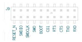
Figure 6: Peripherals connection pin header of EVK-NINA-B1
