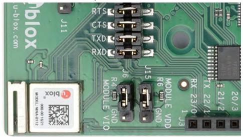
Figure 9: Placement of R4 and R6 (10  $\Omega$  resistors)
