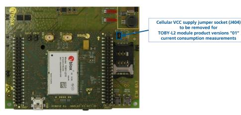
Figure 6: Jumper socket to be removed for TOBY-L2 modules product version "01" current measurement
