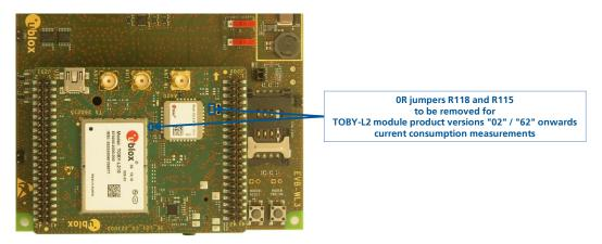
Figure 8: 0R jumpers to be removed for TOBY-L2 modules product versions "02" / "62" onwards current measurement
