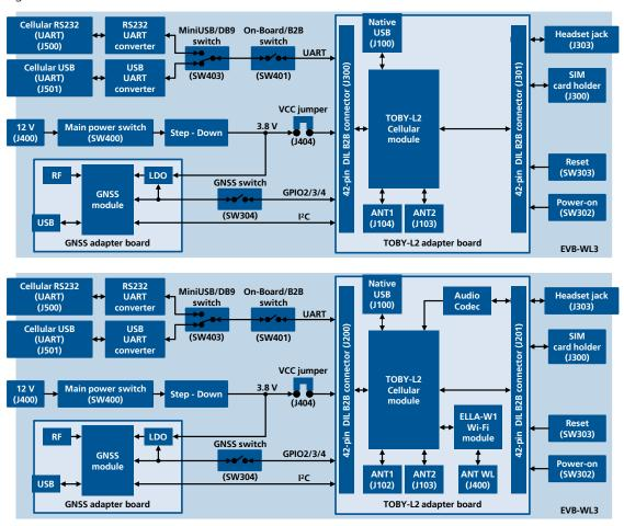
Figure 3: Block diagram of EVK-L2 for TOBY-L2 product versions "01" (top) and "02" / "62" onwards (bottom)
