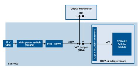
Figure 7: Block diagram of current consumption setup for TOBY-L2 modules product version "01"
