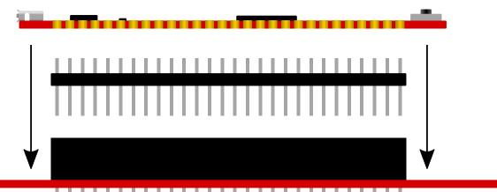
Figure 2-2. Connecting to Curiosity Nano Base for Click boards<sup>™</sup>
