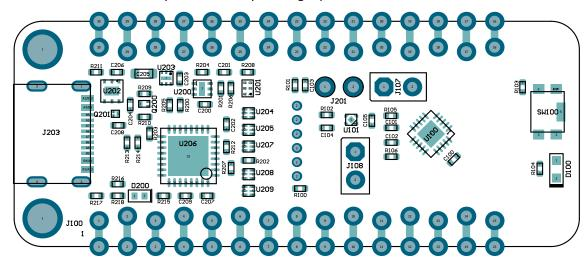
Figure 6-4. PIC18F16Q20 Curiosity Nano Assembly Drawing Bottom
