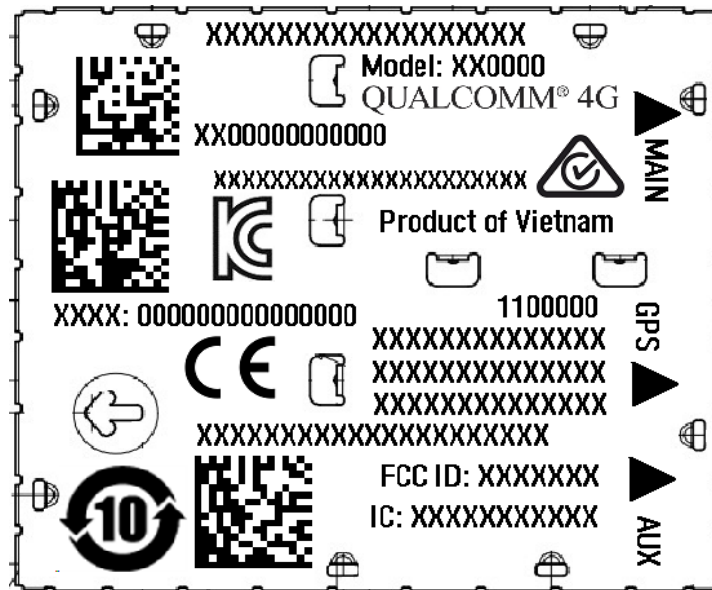
Figure 7-3: Unit Product Marking Example—Laser-etched, Typical Representation (Not to scale. Contents will vary by SKU.)
