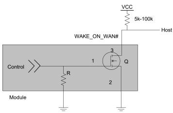
Figure 3-5: Recommended WAKE\_ON\_WAN# Connection
