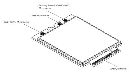
Figure 4-1: Module Connectors
