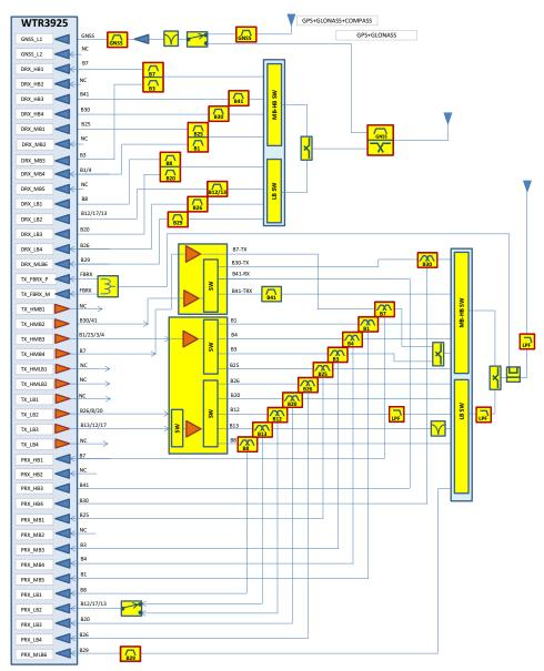
Figure 3-2: Expanded RF Block Diagram
