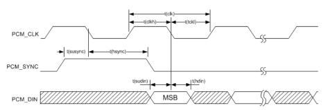
Figure A-3: Module to PCM Codec Timing
