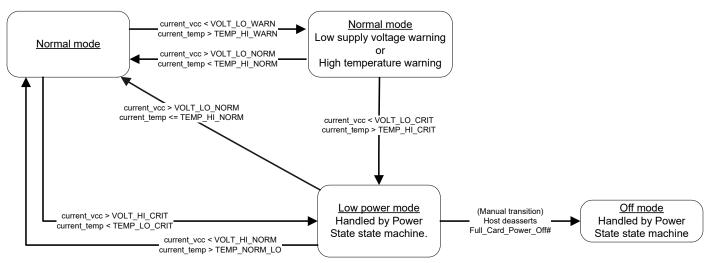
Figure 5-1: Voltage/Temperature Monitoring State Machines
