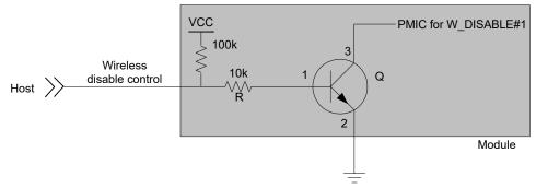
Figure 3-6: Recommended Wireless Disable Connection
