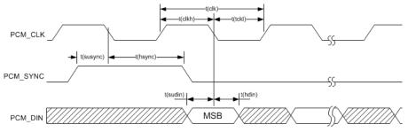
Figure A-2: PCM Codec to Module Timing
