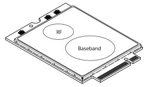
Figure 7-4: Shield Locations (Top View)
