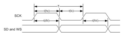
Figure A-4: I2S Transmitter Timing Diagram
