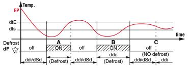
Example: Defrost **A** ends due to reaching of temperature  $\exists \exists E$ , defrost **B** ends at the end of the  $\exists dE$  time as the temperature  $\exists E$  is not reached, defrosting **C** does not take
