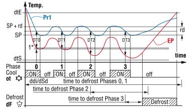
Example "dynamic defrost intervals system" with a reduction ddd = 40% and end defrost by temperature.
