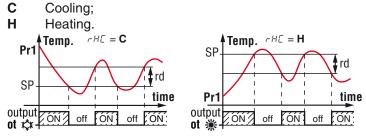
Depending on the function mode programmed with parameter  $r H_{L}^{c}$  the differential is automatically considered by the controller with positive values for a **Refrigeration** control ( $r H_{L}^{c} = C$ ) or negative values for a **Heating** control ( $r H_{L}^{c} = H$ ).
