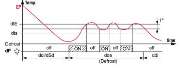
Example of electric defrost with evaporator temperature control: the defrost end after ddE programmed time. During defrost the **dF** output switch ON/OFF to control evaporator temperature in heating mode with set point ddE and 1° differential (Hysteresis).
