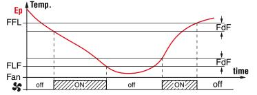
**Note:** It is necessary to pay attention to the correct use of this fans temperature control functions because in the typical application of refrigeration the stop of the evaporator fans stops also the thermal exchange. Remember that the fans functioning can be conditioned by
