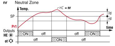
When  $rH\mathcal{L} = \mathbf{nr}$ , the output configured as **ot** operates with a cooling action (like  $rH\mathcal{L} = \mathbf{C}$ ) while the output configured as **HE** operates with a heating action both with the active Set Point (*SP/SPE/SPH*). The intervention differential (rd/rEd/rHd) is automatically assumed by the controller to have positive values for the cooling action and negative values for the heating action. **HC** Cooling and Heating with independent Set Points
