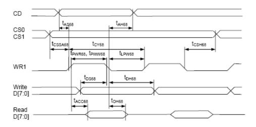
Parallel Bus Timing Characteristics (for 6800 MCU)
