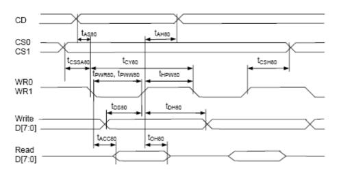
Parallel Bus Timing Characteristics (for 8080 MCU)
