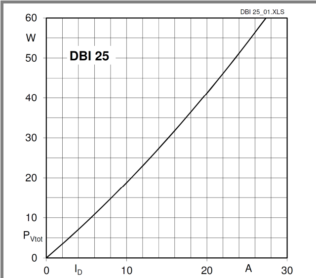
Fig. 3L Power dissipation vs. output current
