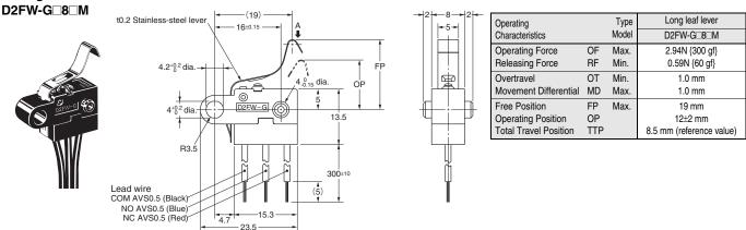
Note1. Unless otherwise specified, a tolerance of  $\pm 0.4$  mm applies to all dimensions. Note2. The operating characteristics are for operation in the A direction ( -).
