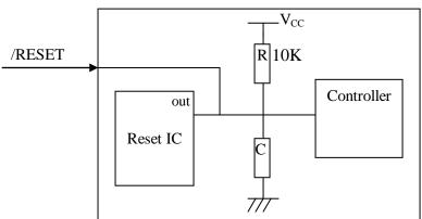
Configuration of Reset-IC peripheral circuit.
