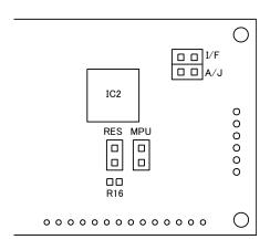
Default setting is no external reset inputs, M68 CPU bus parallel interface and Katakana font. External reset input signal is active when it is low.
