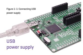
You can supply power to the board with a micro USB cable provided in the package. On-board voltage regulators provide the appropriate voltage levels to each component on the board. Power LED [GREEN] will indicate the presence of power supply.
