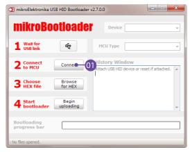
Figure 3-2: USB HID mikroBootloader window
