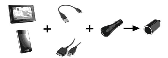
• Connect the plugs to the respective terminals in the car and in the external device.
