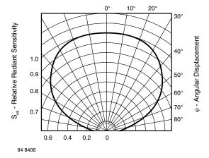
Fig. 7 - Relative Radiant Sensitivity vs. Angular Displacement
