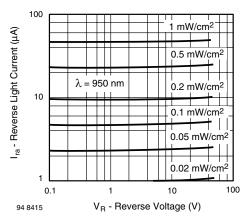
Fig. 4 - Reverse Light Current vs. Reverse Voltage
