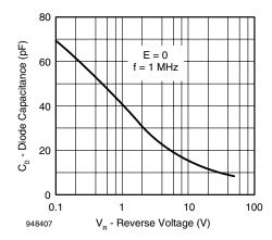
Fig. 5 - Diode Capacitance vs. Reverse Voltage
