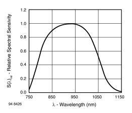
Fig. 6 - Relative Spectral Sensitivity vs. Wavelength
