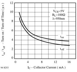
Figure 7. Turn On/Turn Off Time vs. Collector Current
