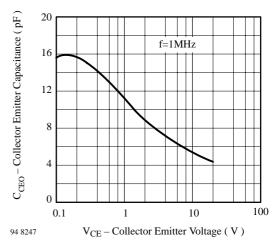
Figure 6. Collector Emitter Capacitance vs. Collector Emitter Voltage
