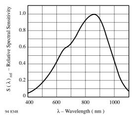
Figure 8. Relative Spectral Sensitivity vs. Wavelength
