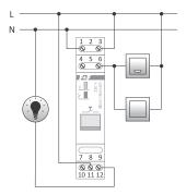
Example of connection with control pulse L
