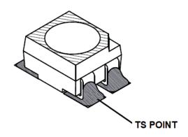
$T_S$  can be easily measured by mounting a thermocouple on the soldering joint as shown in preceding figure, while  $R_{\theta J\text{-}S}$  is provided in the data sheet. Verify the  $T_S$  of the LED in the final product to ensure that the LEDs are operating within all maximum ratings stated in the data sheet.
