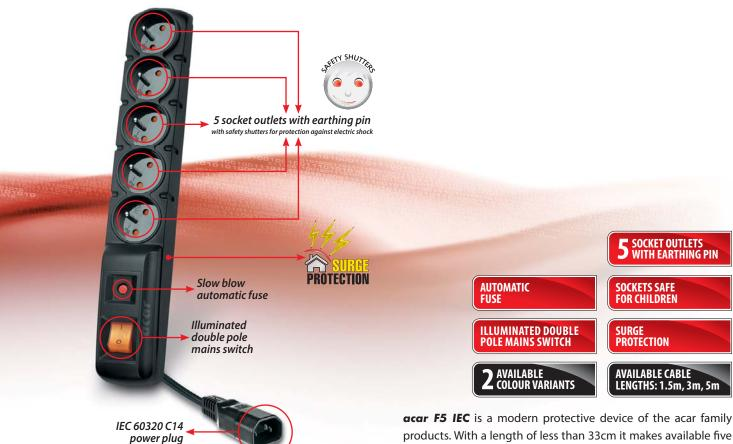
products. With a length of less than 33cm it makes available five sockets outlets with earthing. Application of computer power plug IEC 60320 C14 determines its professional use, and applying of automatic fuse creates the product virtually maintenance-free. High efficiency predisposes the device to become the basic surge protector, which is necessary in every place. Mounting brackets are optional and available from the distributor.
