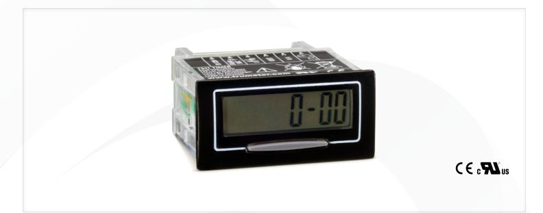
8-digit liquid crystal display timer, self-powered with a 10-year battery life. A compact LCD timer designed for many applications, screw terminals ensure fast wiring. Features include backlighting (external 5VDC supply required), 4 timing modes, timing direction indication and 9mm high digits. High Voltage (HV) version accepts input voltages of 5-110VDC or 10-240VAC.
