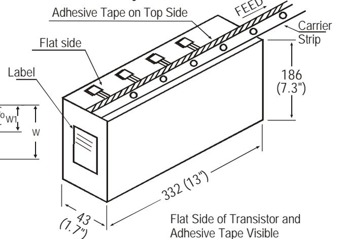
Flat Side of Transistor and Adhesive Tape Visible
