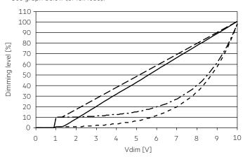
Soft-linear dimming curve 1 % min. to 0 Linear dimming curve 10 % min. to 0 **– – –** Logarithmic dimming curve 1 % min. to 0 Square dimming curve 10 % min. to 0
