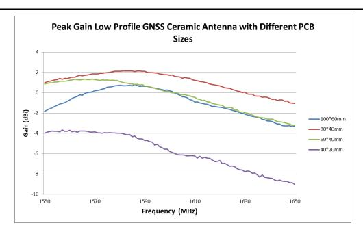
FIGURE 4.3.3 PEAK GAIN OF ANTENNA COMPARISON AT GPS/GALILEO/BEIDOU/GLONASS BAND MOUNTED ON DIFFERENT GROUND SIZES
