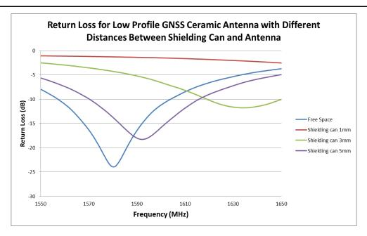
FIGURE 4.2.1 RETURN LOSS OF ANTENNA COMPARISON AT GPS/GALILEO/BEIDOU/GLONASS BAND WITH DIFFERENT DISTANCES BETWEEN SHIELDING CAN AND ANTENNA
