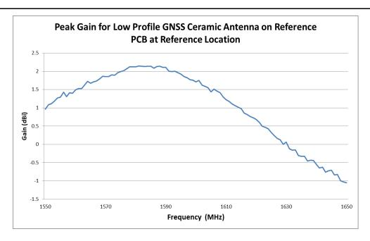
FIGURE 2.4 PEAK GAIN OF ANTENNA AT GPS/GALILEO/BEIDOU/GLONASS BAND ON REFERENCE PCB AT REFERENCE LOCATION IN FREE SPACE
