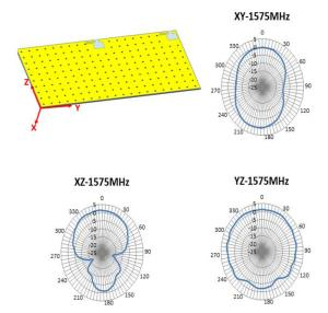
FIGURE 6.2 RADIATION PATTERN OF ATNENNA AT 1575MHZ AT RECOMMENDED LOCATION
