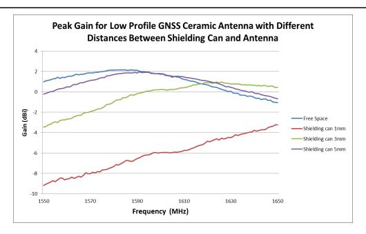
FIGURE 4.2.3 PEAK GAIN OF ANTENNA COMPARISON AT GPS/GALILEO/BEIDOU/GLONASS BAND WITH DIFFERENT DISTANCES BETWEEN SHIELDING CAN AND ANTENNA
