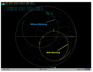
FIGURE 5.4 SMITH CHART OF ANTENNA WITHOUT AND WITH MATCHING NETWORK ON REFERENCE PCB GROUND SIZE AT REFERENCE LOCATION
