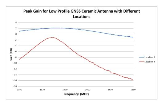
Figure 4.1.3 PEAK GAIN OF ANTENNA AT GPS/GALILEO/BEIDOU/GLONASS BAND AT TWO DIFFERENT LOCATIONS
