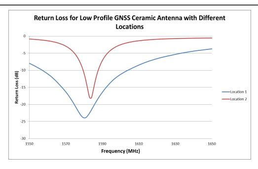
Figure 4.1.1 RETURN LOSS OF ANTENNA AT GPS/GALILEO/BEIDOU/GLONASS BAND AT TWO DIFFERENT LOCATIONS
