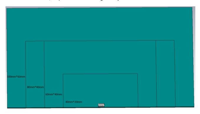
FIGURE 4.3 DIFFERENT GROUND PCB SIZES
