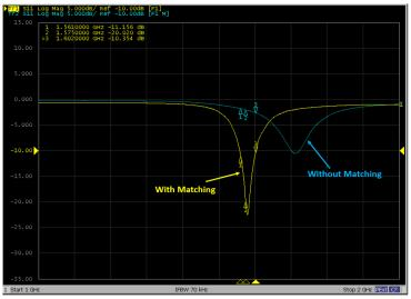
FIGURE 5.3 RETURN LOSS OF ANTENNA WITHOUT AND WITH MATCHING NETWORK ON REFERENCE PCB GROUND SIZE AT REFERENCE LOCATION
