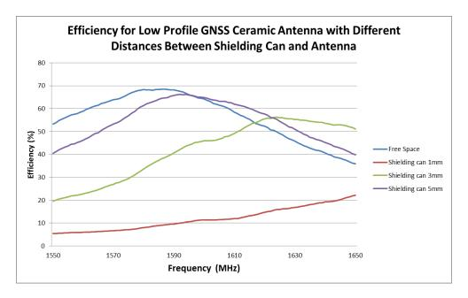
FIGURE 4.2.2 EFFICIENCY OF ANTENNA COMPARISON AT GPS/GALILEO/BEIDOU/GLONASS BAND WITH DIFFERENT DISTANCES BETWEEN SHIELDING CAN AND ANTENNA
