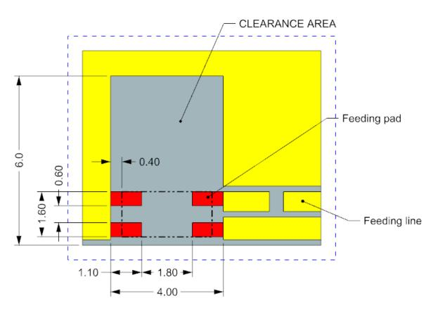
FIGURE 7.5 RECOMMENDED FOOTPRINT ON PCB FOR SOLDERING
