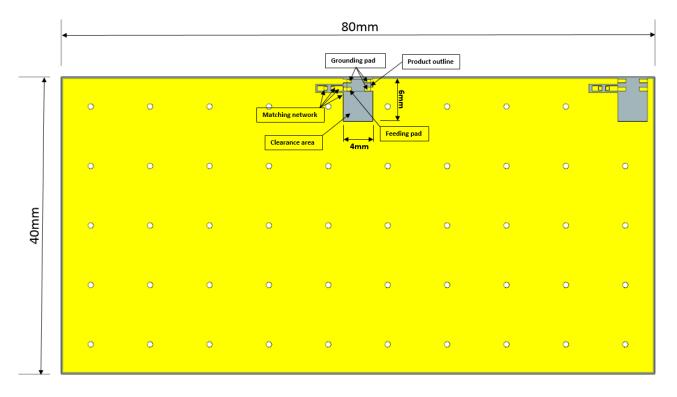
FIGURE 2: REFERENCE PCB LAYOUT
