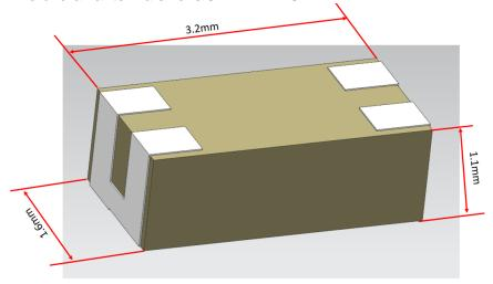
FIGURE 7.2 OVERALL ANTENNA SIZE
