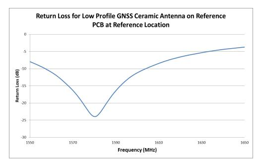
FIGURE 2.2 RETURN LOSS OF ANTENNA AT GPS/GALILEO/BEIDOU/GLONASS BAND ON REFERENCE PCB AT REFERENCE LOCATION IN FREE SPACE
