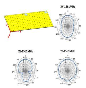
FIGURE 6.1 RADIATION PATTERN OF ATNENNA AT 1561MHZ AT RECOMMENDED LOCATION
