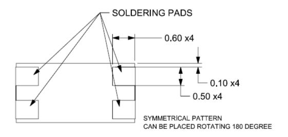
FIGURE 7.4 PADS OF PRODUCT FOR SOLDERING
