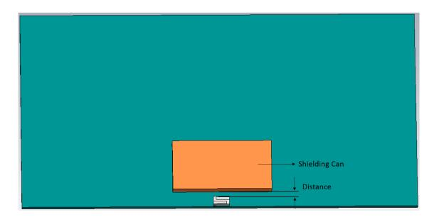
Figure 4.2 SHIELDING CAN FIXED ON REFERENCE PCB
