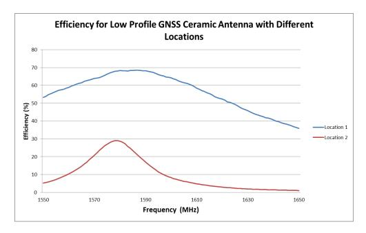
Figure 4.1.2 EFFICIENCY OF ANTENNA AT GPS/GALILEO/BEIDOU/GLONASS BAND AT TWO DIFFERENT LOCATIONS
