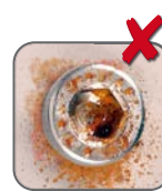
STAINLESS STEEL + NO STAINLESS STEEL = RUST
