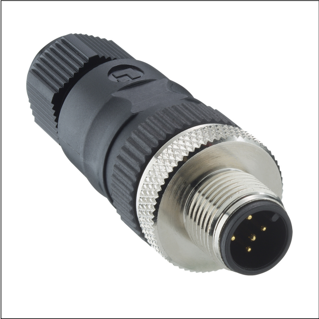
M12 connector, male, field-attachable, with screw clamps, straight, A-coded, IP67
