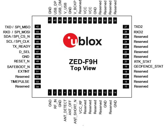
Figure 3: ZED-F9H-01B pin assignment
