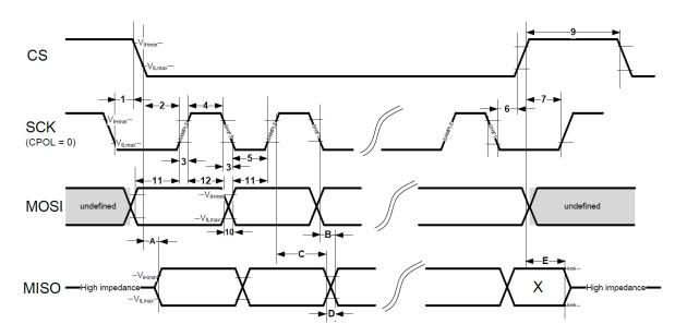
Figure 4: ZED-F9H-01B SPI specification mode 1: CPHA=0 SCK = 5.33 MHz
