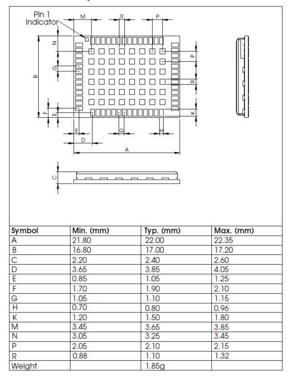
Figure 6: ZED-F9H-01B mechanical drawing
