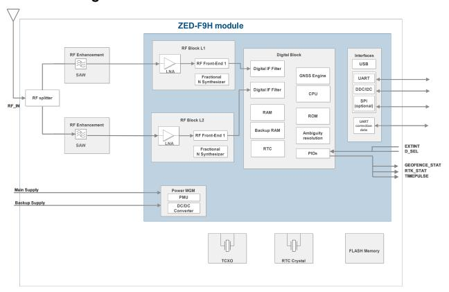
Figure 2: ZED-F9H-01B block diagram
