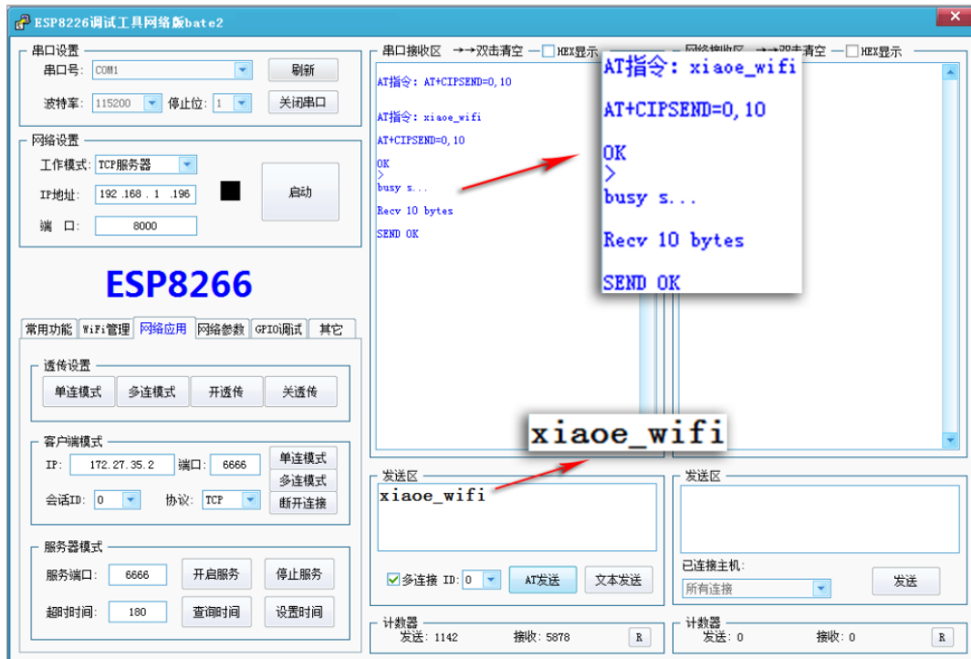
Figure 4-25 Test Software - Data Transmission (Station Mode)
