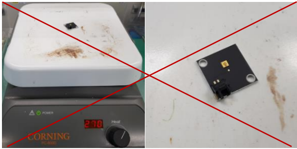
FIG 9. Do not use a hot plate to mount led-package onto PCB. A reflow oven is recommended.
