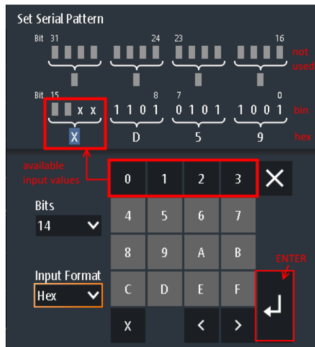
Figure 2-16: Pattern editor for 14-bit pattern in hexadecimal format
