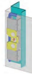
Position 2 - After the door is opened, cam is rotated 90° with a screwdriver
