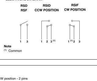
RSDSPST: Single pole, open switch in CCW position - 2 pinsRSFSPST: Single pole, open switch in CW position - 2 pinsRSIDSPDT: Single pole, changeover switch in CCW position - 3 pinsRSIFSPDT: Single pole, changeover switch in CW position - 3 pins
