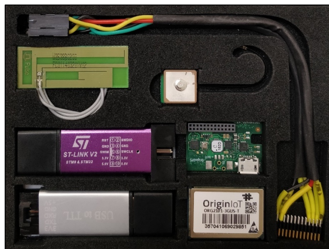
Figure 1. OriginIoT™ Application Kit Contents
