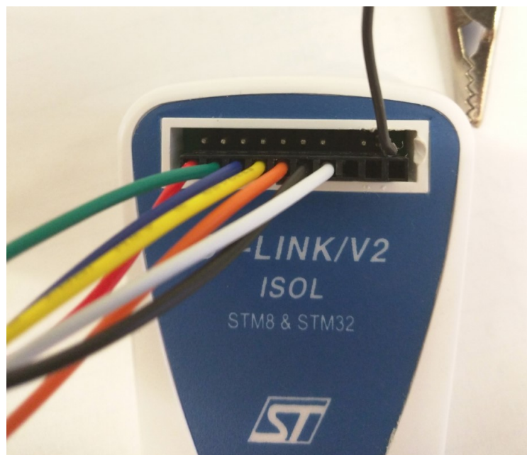
Figure 33: ST-Link plug orientation
