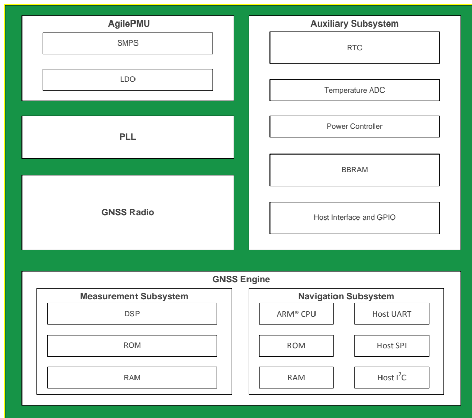
FIGURE 2 – SiRFstarV™ 5e GNSS SoC BLOCK DIAGRAM
