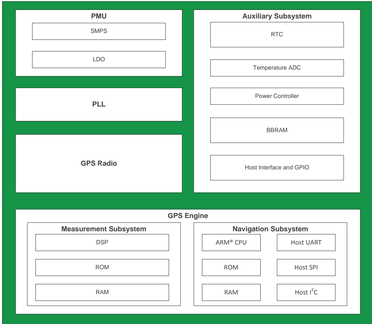
FIGURE 2 – SiRFstarIV™ GSD4e GPS SoC BLOCK DIAGRAM
