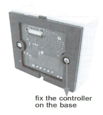
(4) use your hand gently pull down the cable seat lock according to step 2, plug the cable into cable seat, press the lock, and mount the cable of panel on the base, as shown below:
