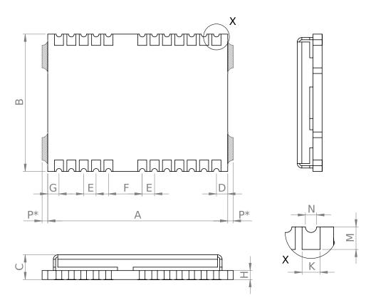
Figure 4 NEO-8Q mechanical drawing
