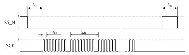
Figure 3: SPI timing diagram
