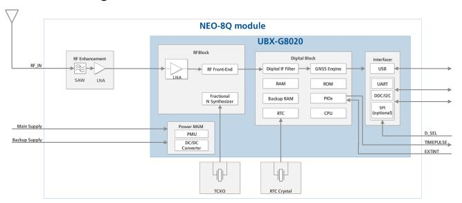
Figure 1: NEO-8Q block diagram
