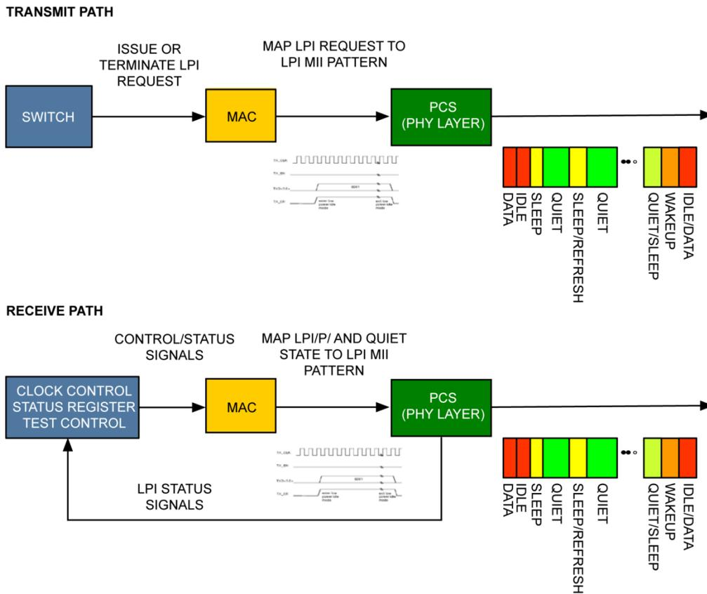
Figure 5. EEE Transmit and Receive Signaling Paths
