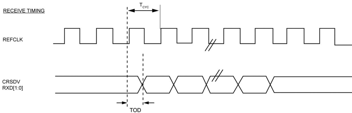
**Figure 20. RMII Timing – Data Transmitted to RMII**
