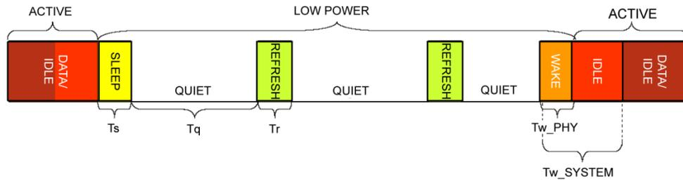
Ts = THE PERIOD OF TIME THAT THE PHY TRANSMITS THE SLEEP SIGNAL BEFORE TURNING ALL TRANSMITTERS OFF,  $200 \leq T_s \leq 220$  USED IN 100BASE-TX.
