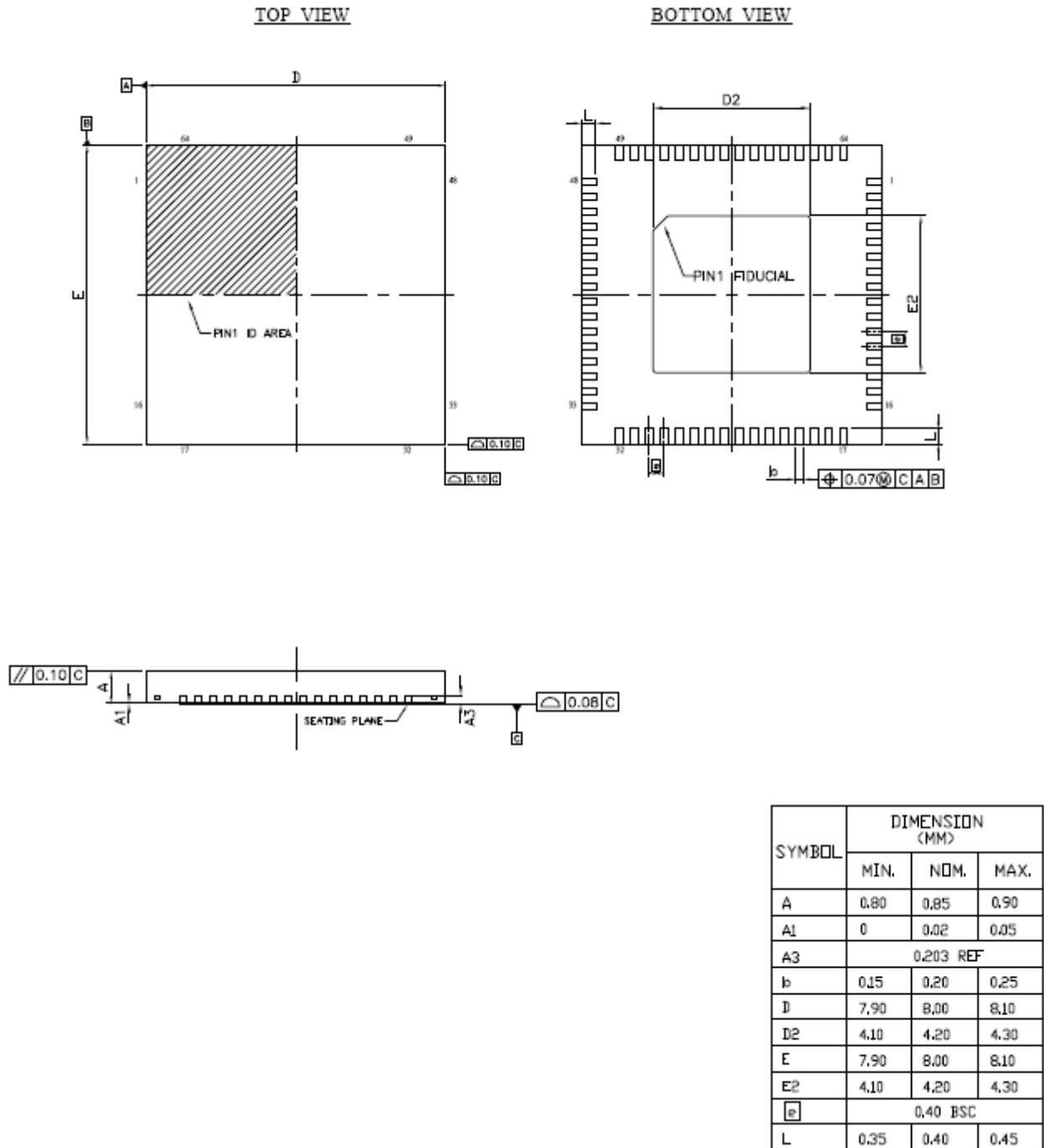
Figure 27. 64-Pin (8mm x 8mm) QFN Package
