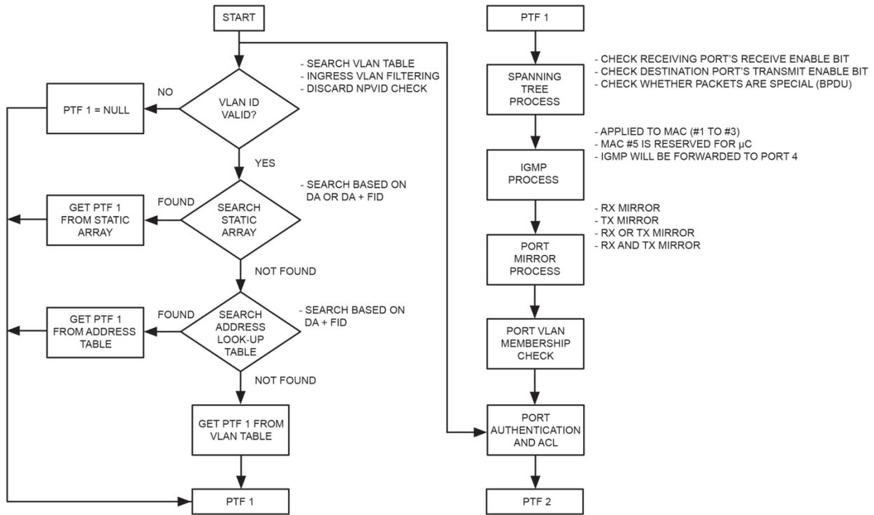
Figure 4. Destination Address Lookup and Resolution Flow Chart
