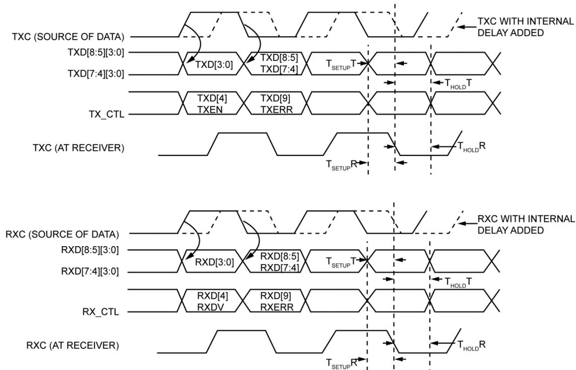
Figure 14. RGMIITiming v2.0 Specification (Figure3-Multiplexing and Timing Diagram)
