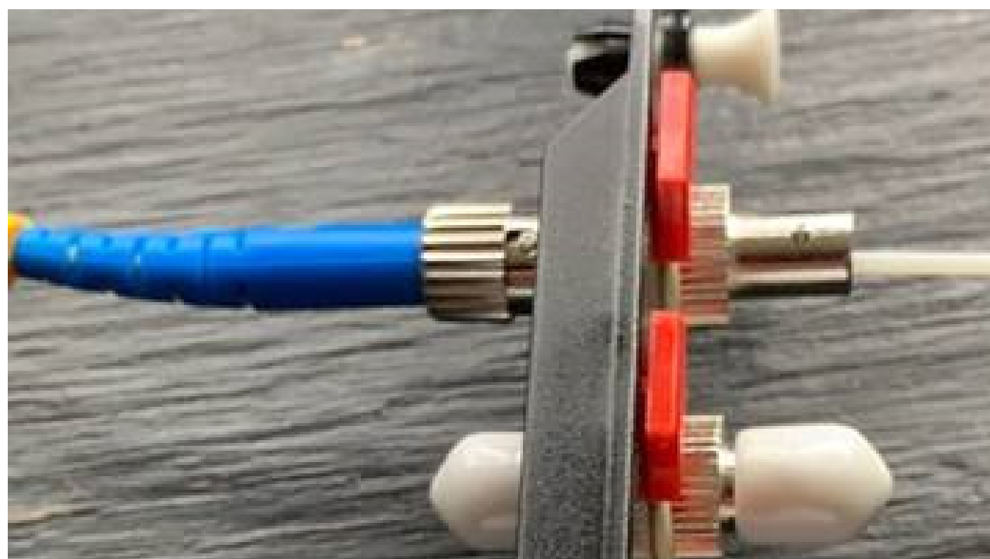
Cleaning ST/UPC in Adapter
