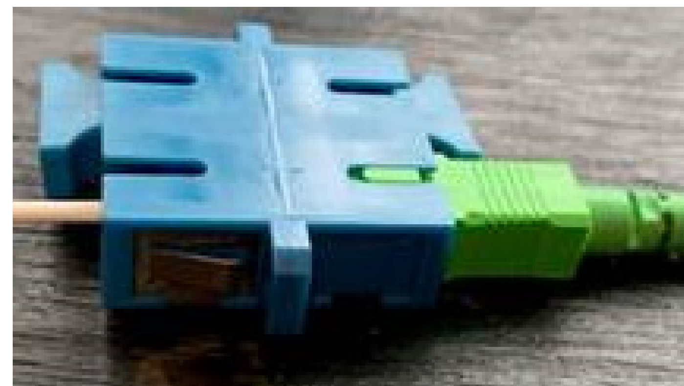
Cleaning SC/APC in Adapter
