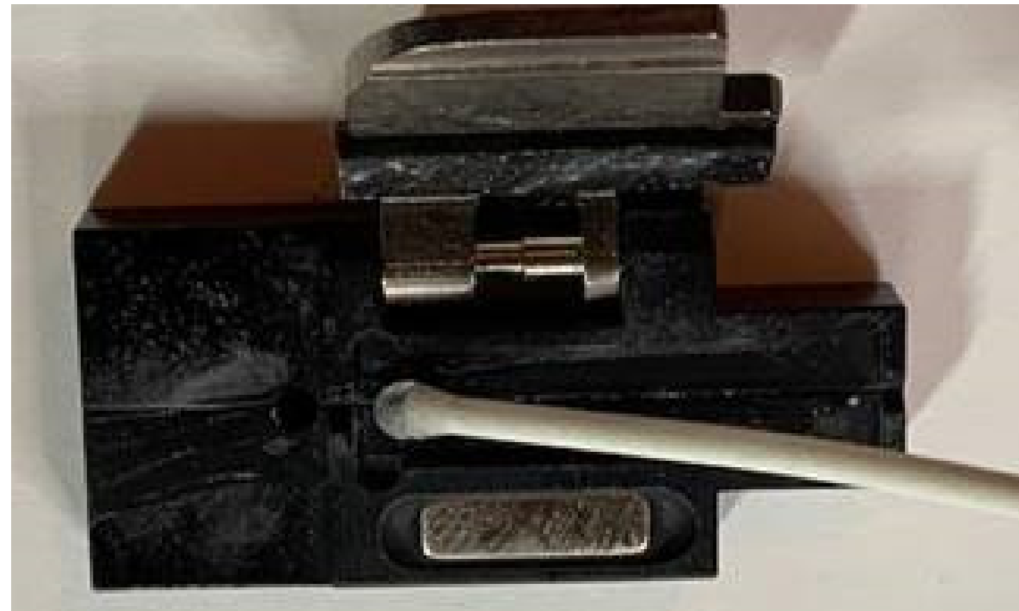
2. Swab used to wipe the V groove and around the inner channel surface.
