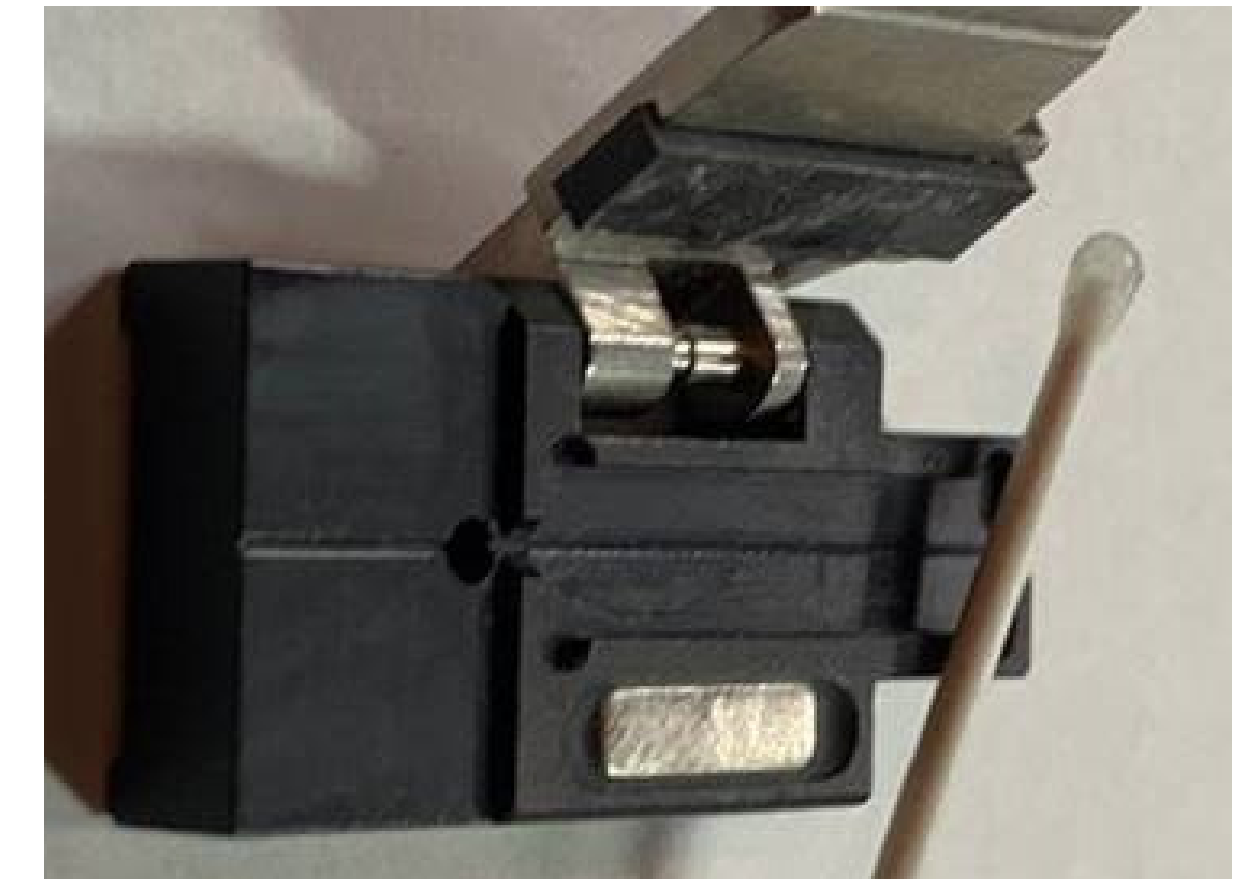
3. End result after wiping the fiber holder using a single stick. The V groove is clean and the area around it are clean. No scratches or residue streaks whatsoever.
