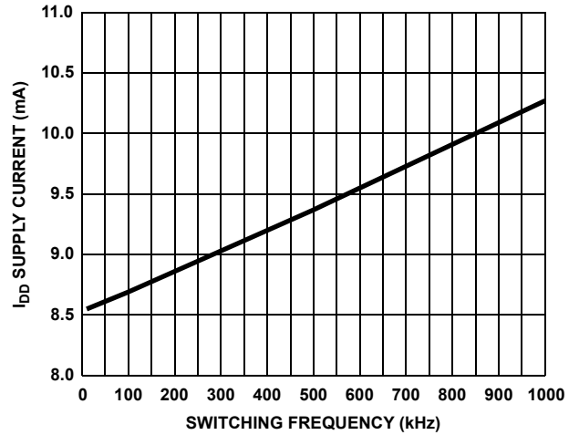
FIGURE 5. I_{DD0} , NO-LOAD I_{DD} SUPPLY CURRENT vs FREQUENCY (kHz)
