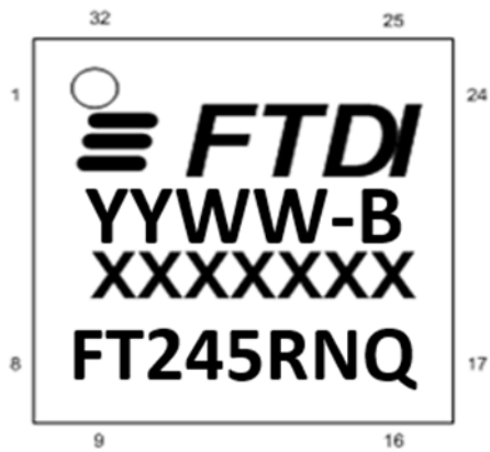
Figure 5-4 Package Markings – FT245RNQ
