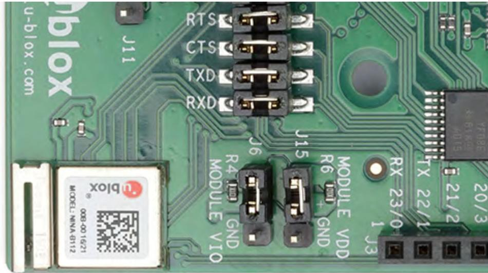
**Figure 9: Placement of R4 and R6 (10  $\Omega$  resistors)**
