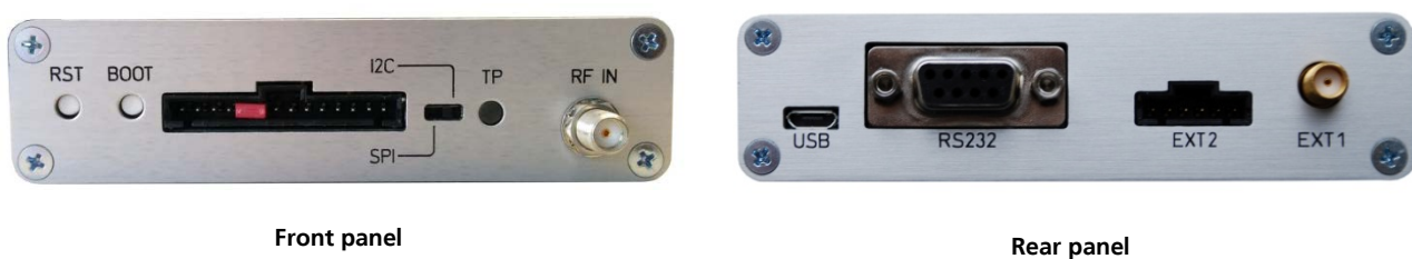
Figure 2: EVK-M8F-0-01 evaluation unit – front and rear panels
