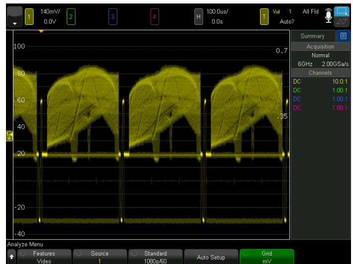
Figure 45. Triggering on a 1080p/60 signal.
