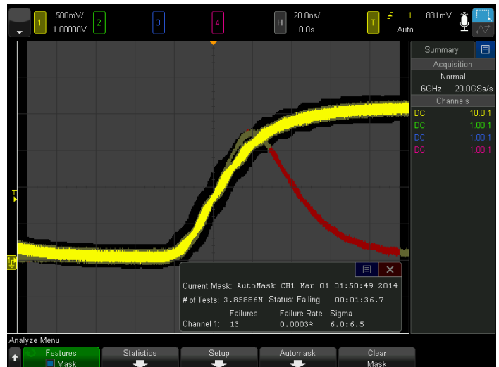
Figure 40. Limit testing of infrequent glitch.
