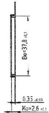
**Figure 4:** tape and reel drawing (in mm)
