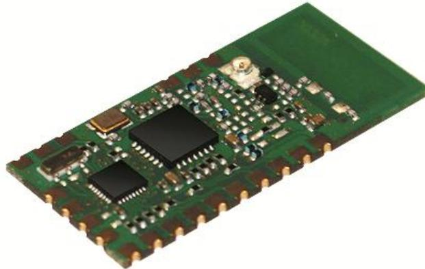
XTR-8LR-ENC is a transceiver based on LoRa™ modulation able to guarantee very long range communication ( 8 Km line of sight ), high interference immunity , very high sensitivity and very low current consumption.
